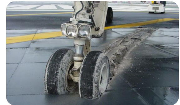
EMASMAX - the premanufactured EMAS block system (runwaysafe.com)
